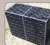
The infiltration trench featured here is filled with plastic containers that resemble milk crates. During installation, the containers are stacked and placed side by side, then wrapped with geotextile material to keep soil from entering the storage area. Runoff from the roof downspouts is diverted to the trench, and is stored in the fabric-wrapped containers. Over time, water seeps through the fabric into the ground to recharge the groundwater supply.
